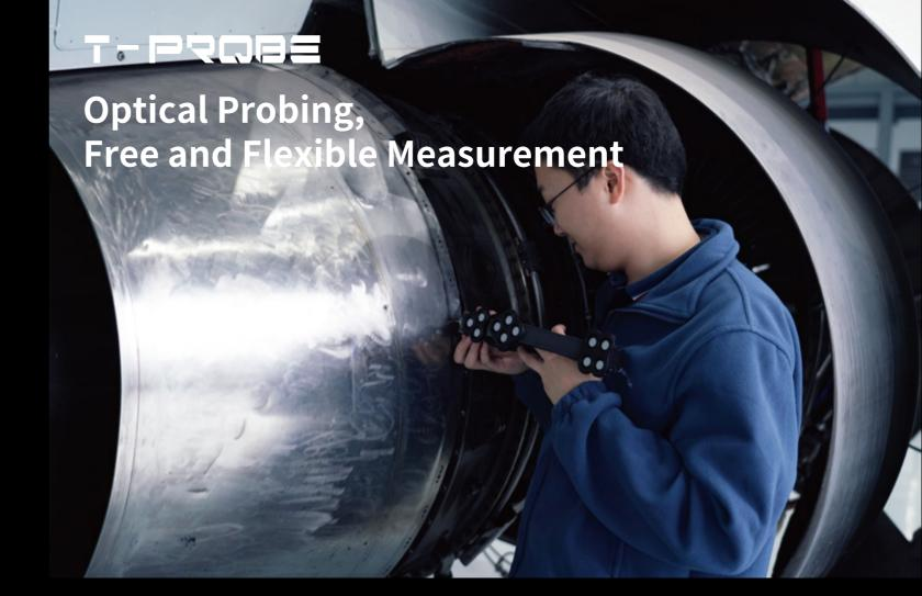
T-Probe is a portable CMM probing system that comes with the i-Tracker to obtain dimensions of features, such as reference holes and hidden points. It can be widely used in the measurement of fixtures, stamping parts, and marking for actual machining allowance.
